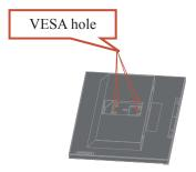
Step 5: Attach the LCD display to the wall, following the instructions in the wallmounting kit. For use only with UL/GS Listed Wall Mount Bracket with minimum weight/load: 8kg
